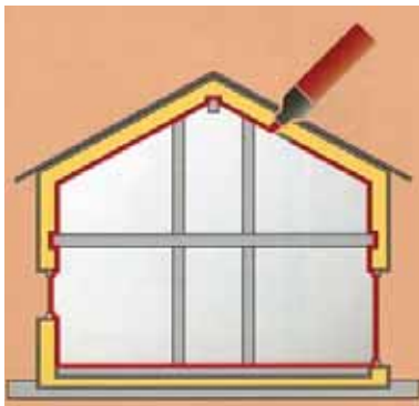
Continuous Airtight Membrane. Source: Passivhaus Institut, Germany
