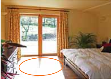
Photo depicting how the low winter sun enters the room below the overhang/awning/balcony. Source: MosArt Architecture.
